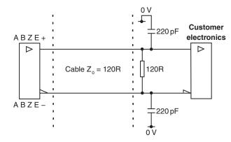
Standard RS422A line receiver circuitry The capacitors are recommended for improved noise immunity
