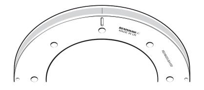
**NOTE:** The *IN-TRAC*<sup>™</sup> reference mark is integrated in the scale, radially aligned with the centre of the mounting hole to the left of the 'Renishaw' logo within ±0.5 mm. No external actuators or physical adjustments are required. For REXT20, the second reference mark is 180° from the first.
