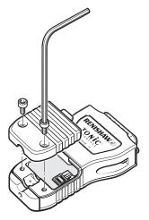
2. Taking care not to touch the pins, plug the connector into the socket in the interface, ensuring correct orientation as shown.
