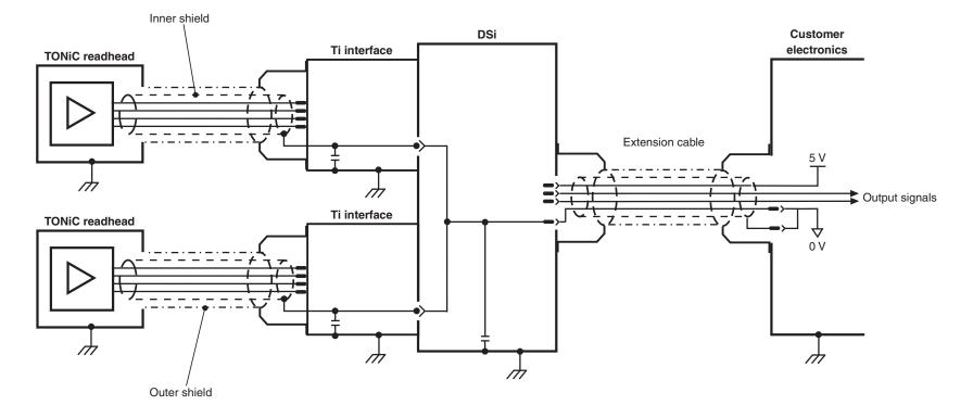
**IMPORTANT:** The outer shield should be connected to the machine earth (Field Ground). The inner shield should be connected to 0 V at the receiving electronics only. Care should be taken to ensure that the inner and outer shields are insulated from each other. If the inner and outer shields are connected together, this will cause a short between 0 V and earth, which could cause electrical noise issues
