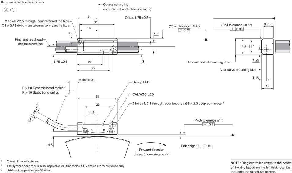
The recommended thread engagement is 5 mm (7.5 mm including counterbore) and the recommended tightening torque is between 0.25 Nm and 0.4 Nm.
