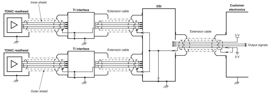
**IMPORTANT:** The outer shield should be connected to the machine earth (Field Ground). The inner shield should be connected to 0 V at the receiving electronics only. Care should be taken to ensure that the inner and outer shields are insulated from each other. If the inner and outer shields are connected together, this will cause a short between 0 V and earth, which could cause electrical noise issues
